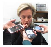
Figure 1. The experimental set-up with the recording devices (iPhone 5 and 6s, Samsung Galaxy S5, head mounted microphone) and the plastic stick that measured 4 cm from the mouth to the microphones.
